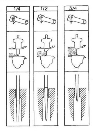
If you look closely at the gap between the jet needle and main nozzle which contains jet needle, you can see if the throttle opens widely, which means the projecting part has withdrawn.
