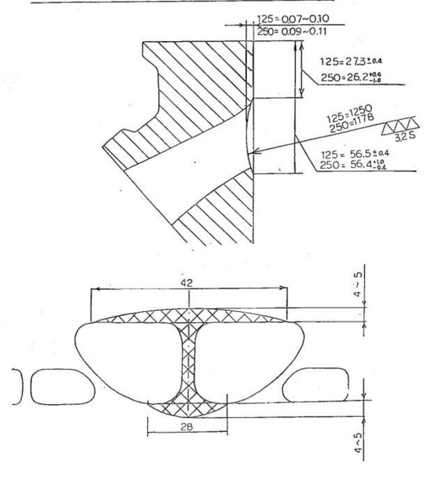
These modifications mentioned enable a considerable improvement in power output. However, it should be understood that these modifications will greatly sacrifice the durability of the parts, especially crankshaft and crank case. Therefore, interval in replacement is critical. Service life of 250 crank is 1,000km and crankcase is 2,000km; same of 125 crank is 500km for your guidline.
