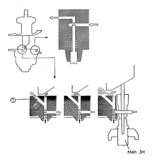
If the throttle valve is slightly open, since the least pressure part is still closer to the engine than the bypass hole, fuel would not discharge from the bypass hole. This would prevent the air-fuel mixture from being too rich due to less air flow from the throttle valve caused by air flowing backwards at the closed or slightly open throttle valve.
