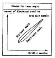
Sometimes the changing linesrepresent the mixture conditions, when the line lowered, less gasoline is discharged for the throttle valve opening, that is, thin air-mixture.
