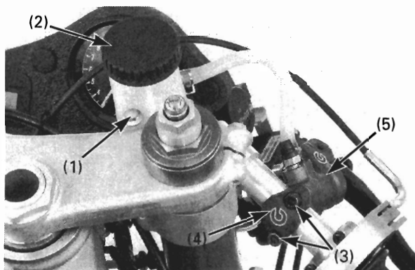
(1) BOLT (2) RESERVOIR (3) BOLTS (4) HOLDER (5) MASTER CYLINDER
