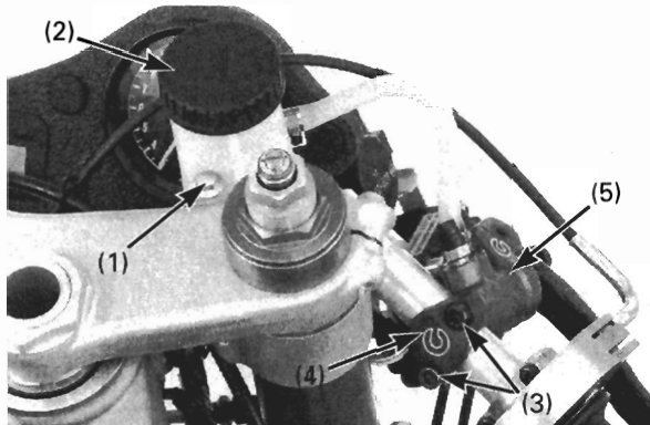
(1) MASTER CYLINDER (2) UP MARK (3) BOLTS
