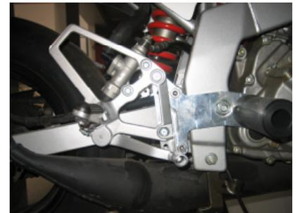
8. Install the plastic frame sliders using the two 10mm x 35mm bolts. A low strength thread lock agent is recommended. Tighten the bolts to a torque of 25 ft-lb. The two pictures on the right show the frame sliders properly installation.
