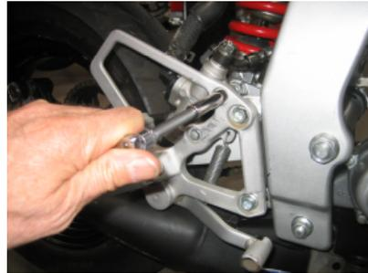
2. Remove both the left and right foot Peg mounting brackets. Remove the nut from the swing arm pivot bolt.
