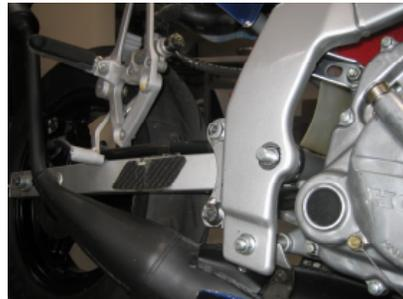
3. Remove the swing arm pivot bolt from the swing arm by pushing it out using a rod (or bolt). The rod will keep the swing arm in position when the pivot bolt is removed from the other side.
