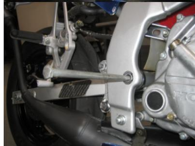
4. Insert the swing arm pivot bolt through the left slider base and into the swing arm pivot. Align the swing to allow the bolt to pass through and out the other side.
